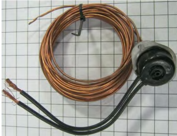
Image 4-6 – Grain column over-temp switch
