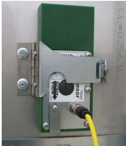
Image 4-9 – Incoming moisture sensor
