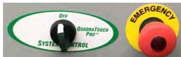
Image 3 – System Control & Emergency Stop switches
