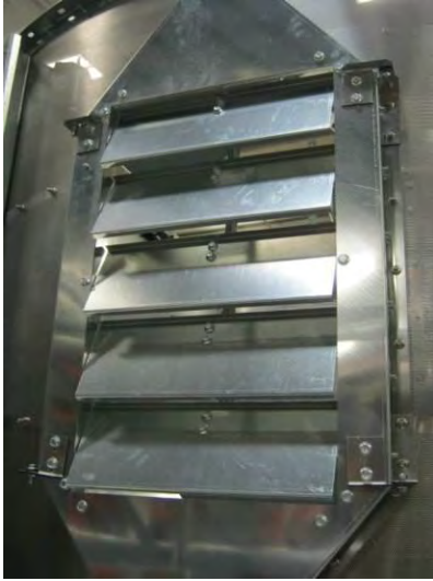
Image 17 – Louvers on door
