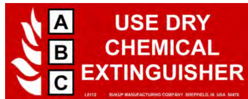
Label #L5112 – Place near main power panel.
