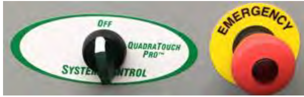
Image 2-1 – System Control switch, Emergency Stop button
