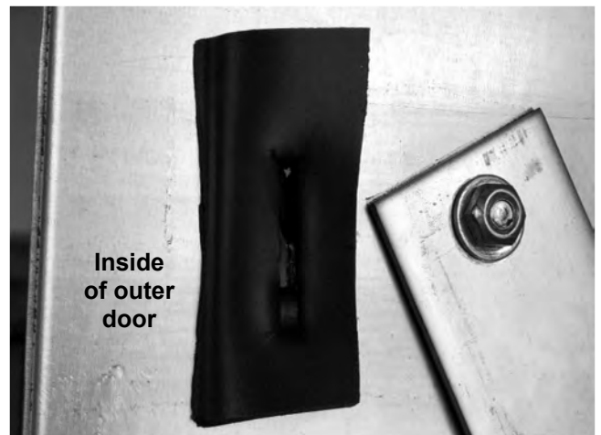
Image 2 – Foam sealant (K6843) on inside of door
