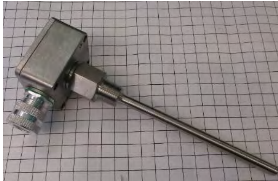
Image 4-10 – Single-point grain temp sensor
