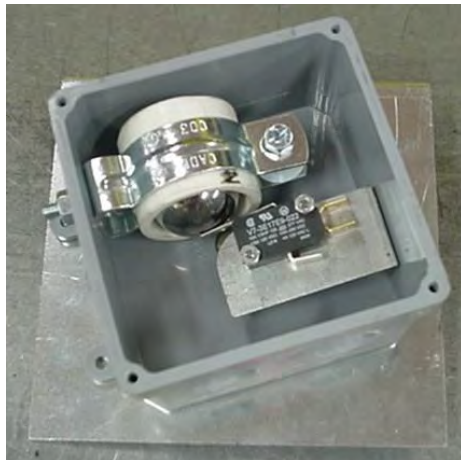
Image 5-2 - Grain level ball switch
