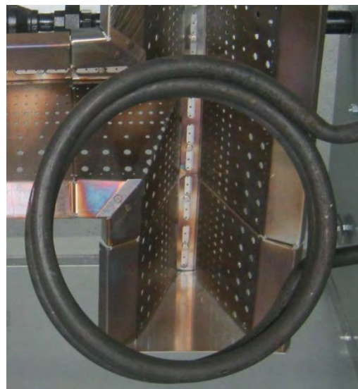
Images 4-21 & 4-22 – Vaporizer coil (shown on octagon burner, left, and on H burner, right)
