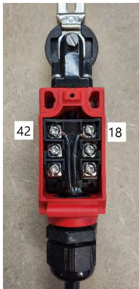
Image 4-18 – Grain discharge box interlock switch
