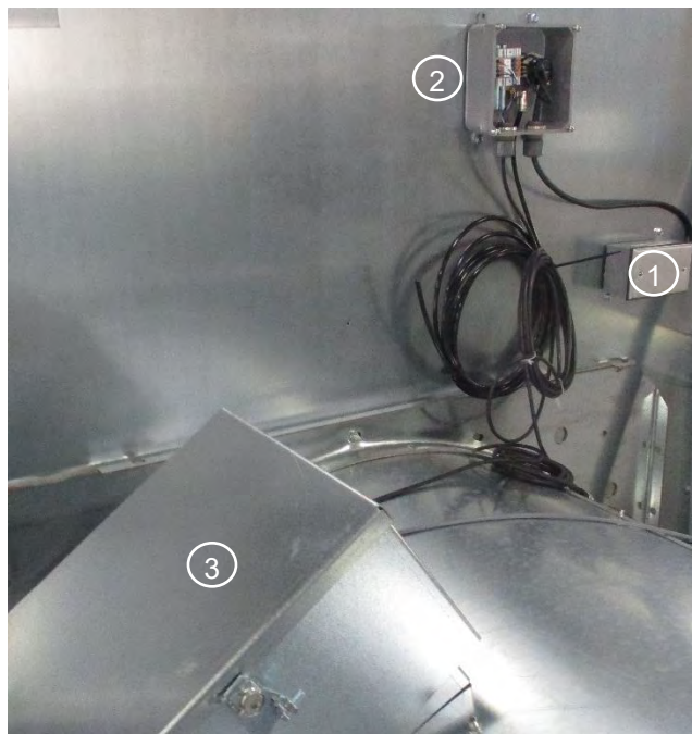
Image 5-13 – Locations on axial dryer of plenum temp sensor RTD, plenum over-temp switch & heater housing high-limit switch
