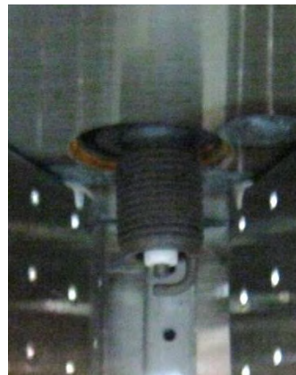
Image 4-20 – Spark plug (shown on H burner)
