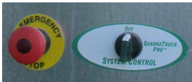
Image 3 – Emergency Stop & System Control switches
