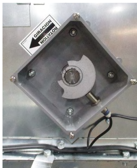
Image 23 – Meter roll proximity switch
