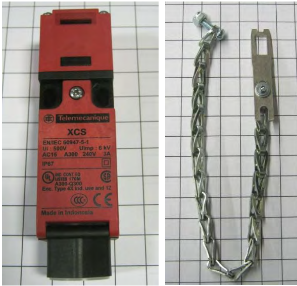
Images 5-6 & 5-7 – Interlock switch (left) & key w/ chain (right)
