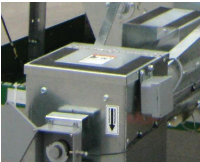
Image 27 - Unload auger service door
