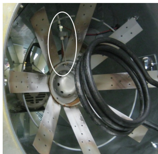
Image 11 - Starfire burner for 28" fan
