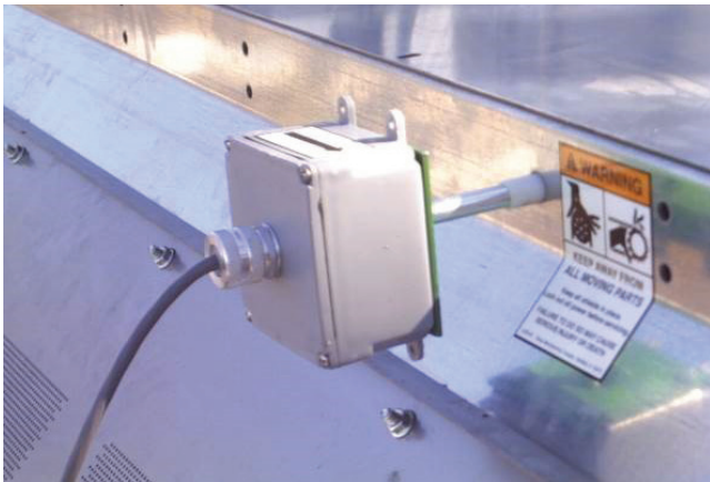
Image 22 - Paddle switch box in operating position
