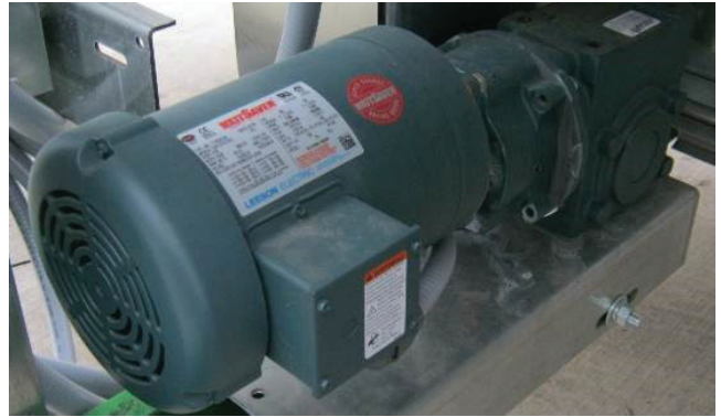
Image 24 - Meter roll motor
