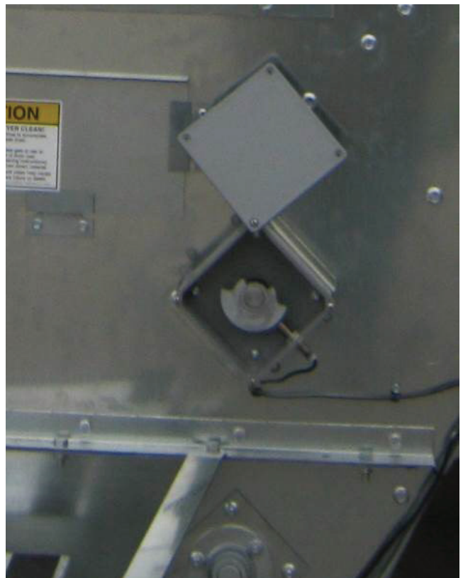
Image 25 - Meter roll proximity switch
