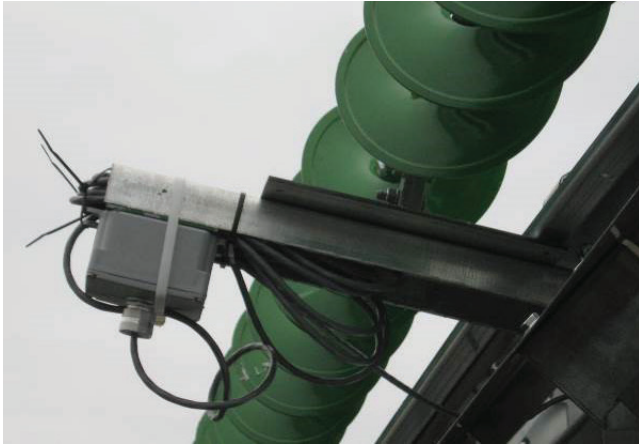
Image 21 - Paddle switch box in shipping position
