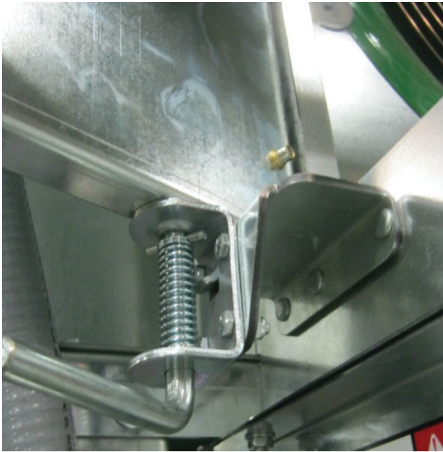
Image 3-5 - Spring pin on intake door
