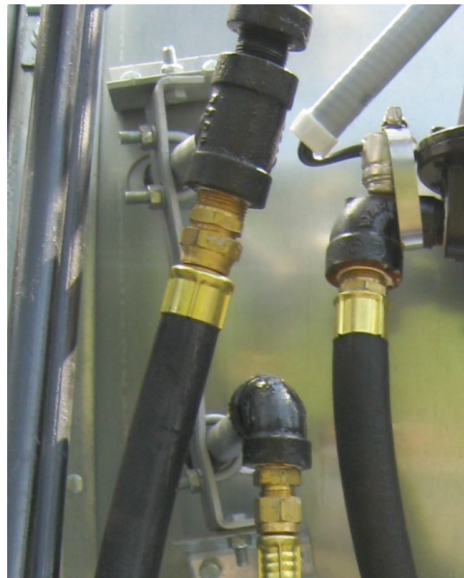
Image 3-1 - Vaporizer adjustment bracket on axial-fan dryer
