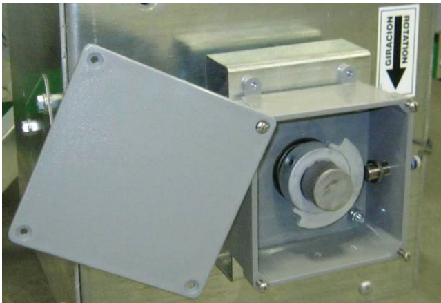
Image 18 - Unload proximity switch
