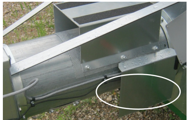
Image 20 - Discharge moisture sensor location
