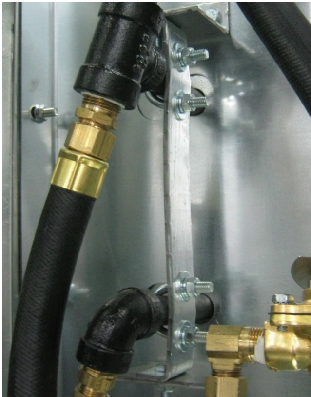
Image 3-2 - Vaporizer adjustment bracket on centrifugal-fan dryer
