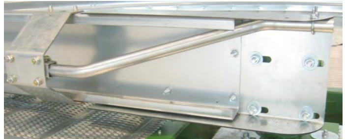
Image 6 – Conduit mounted on sweep backboard
