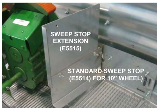
Image 2 – Sweep stop extension added for use with 17" drive wheel
