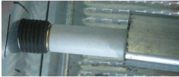
Image 8 – Alignment rod in torsion bar
