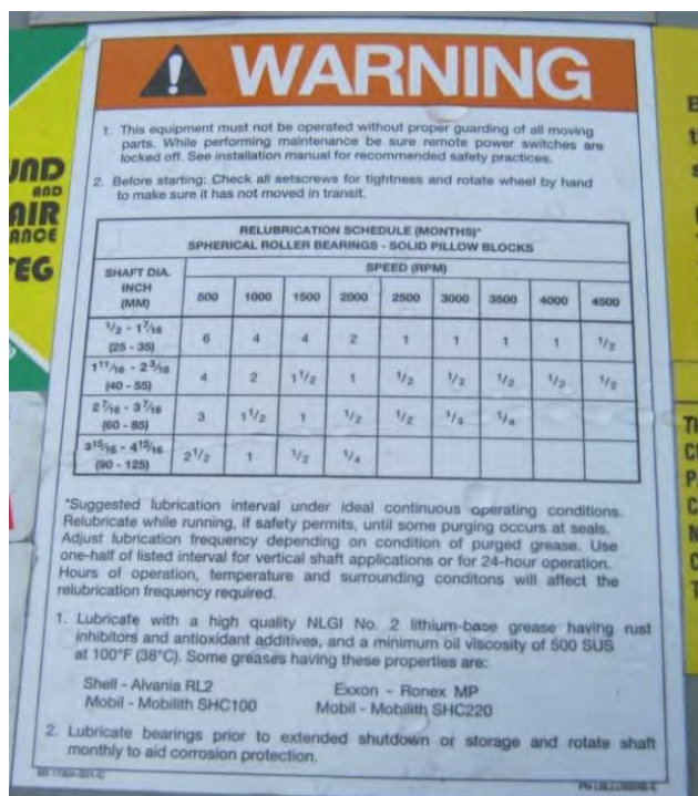
Image 3-2 – Twin City Fan & Blower lubrication sticker
