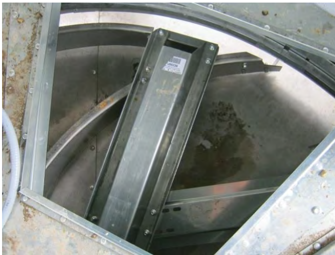
Image 14 shows rotor arm and scraper (curved) of unload.
