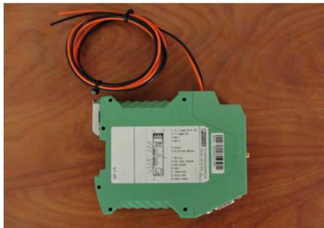
4. Connect the GSM modem to the PLC with the Serial Interface Cable as shown.
