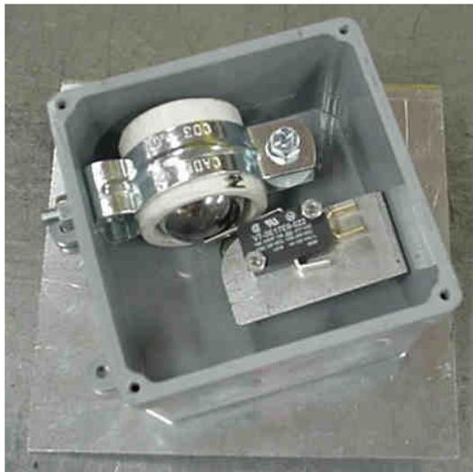
Image 4-3 – Grain discharge chute switch
