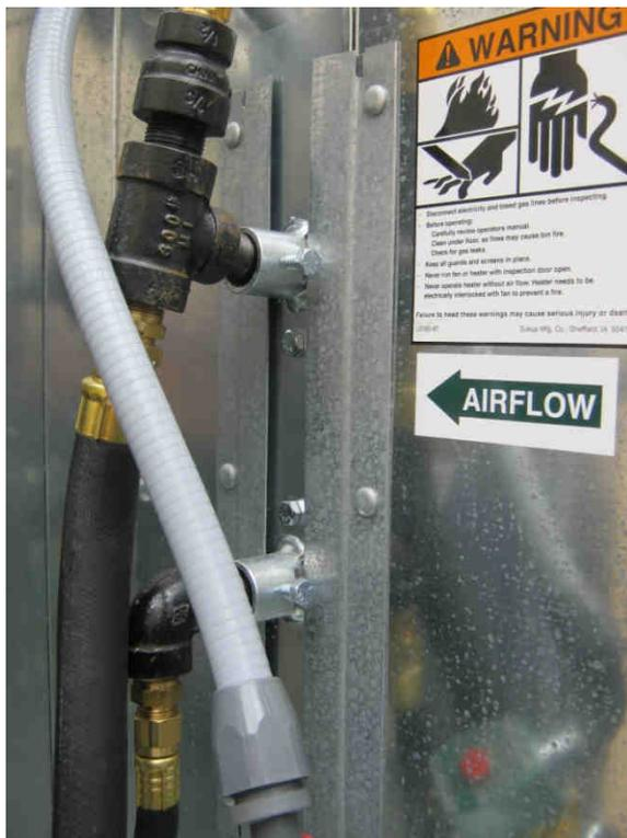
Selecting the Dry Fire / Test Mode is required to operate the dryer's fan and heater when there is no grain in the dryer. After the dryer has been allowed to run and the plenum temperature has stabilized, the vaporizer outlet (top) should be warm but not hot to the touch.
