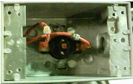
Figure 1.4b: Vapor Over-Temperature Switch
