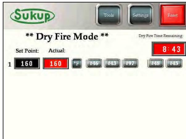
Lastly, “Dry Fire” will conclude after the timer has expired, and the fans and heaters will automatically turn off.
