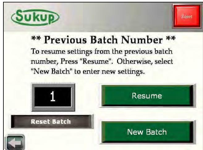
After pressing “New Batch” the user will select a drying temperature.
