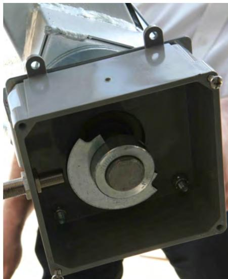
Image 16 shows unload auger proximity switch and rotating target mounted on jump auger
