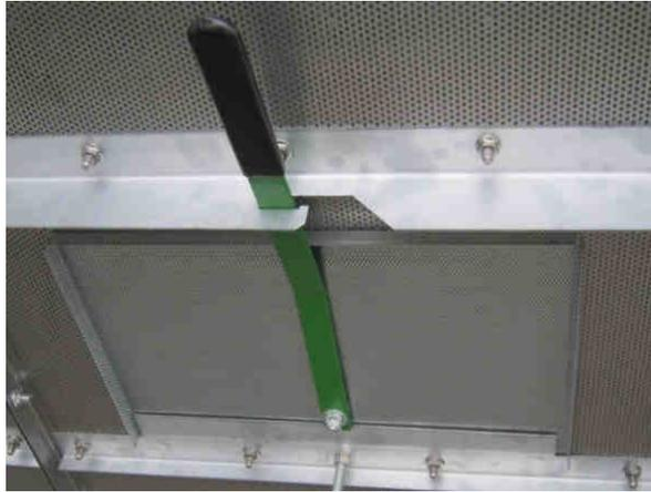
Image 4-34 – Grain column outside cleanout door handle
