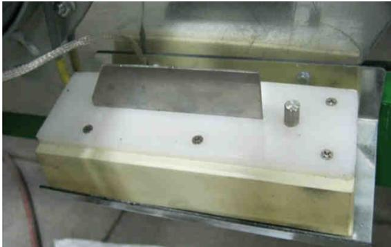
**Image 4-29 – Discharge moisture sensor flag and tube**
