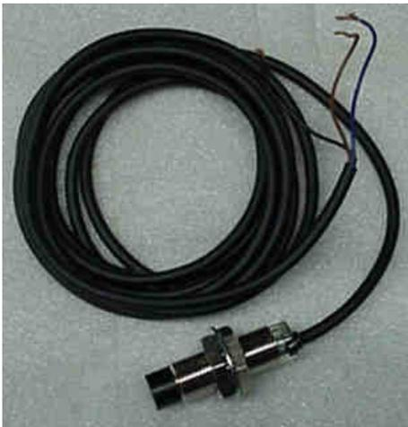
Figure 1.8b: Metering Roll Proximity Switch
