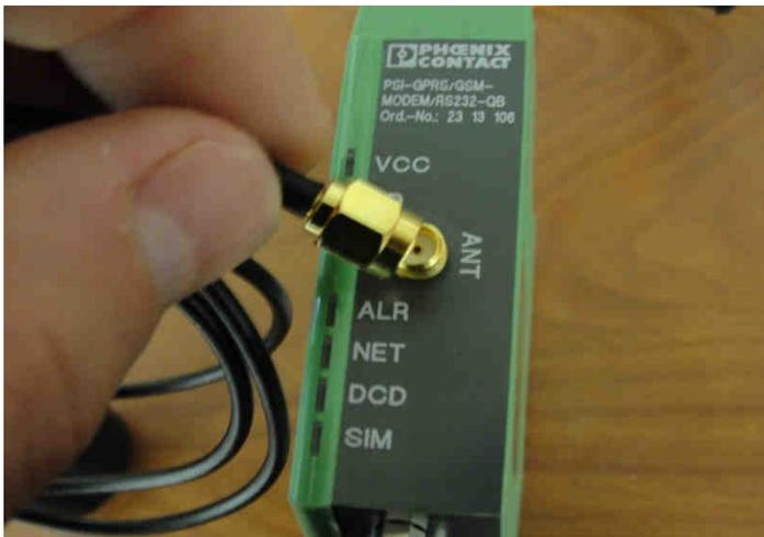
7. You are finished. When you power up, you will see the VCC light flashing. After it has started up, the modem will search for a GSM signal. If it finds a signal, you will see a steady flashing or solid light on the NET light (after a couple of minutes). If the NET light is not lit, the SIM card was not properly activated, or there is no GSM signal. You may have to try a different GSM provider if this is the case.
