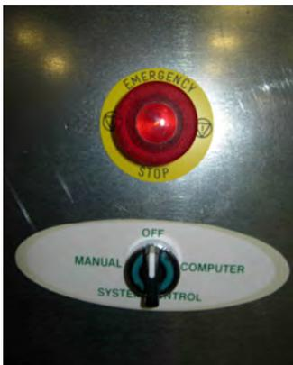
**Image 23 – Emergency stop button and system control switch**
