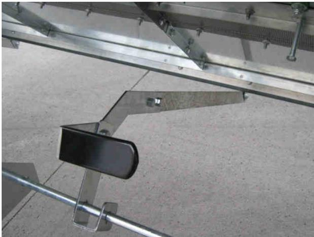
**Image 4-32 – Unload auger outside access/cleanout door handle**
