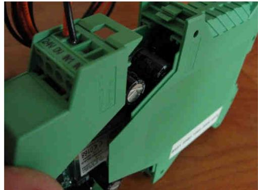
2. Mount GSM modem onto DIN Rail. The modem should be mounted in power box or auxiliary box.
