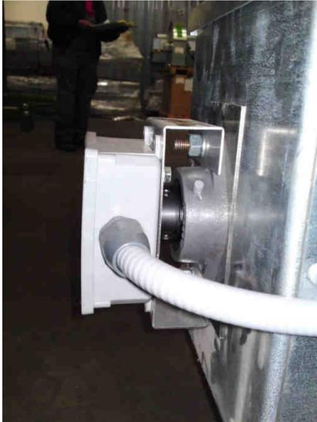
**Image 4-5 – Unload auger proximity switch**
