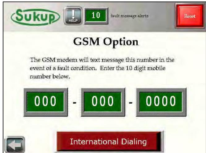
If dialing outside of North America, you may need to change the band setting of the GSM modem. Touch the "Help" button to show band setting options.
