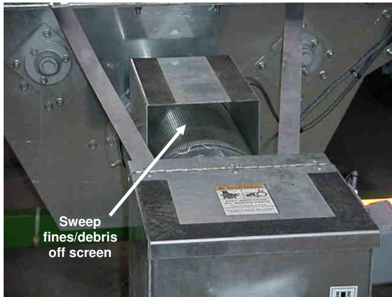
Image 4-27 – Grain discharge chute screen
