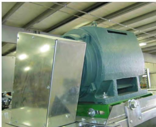
Image 39 – Fan motor and drive shield
