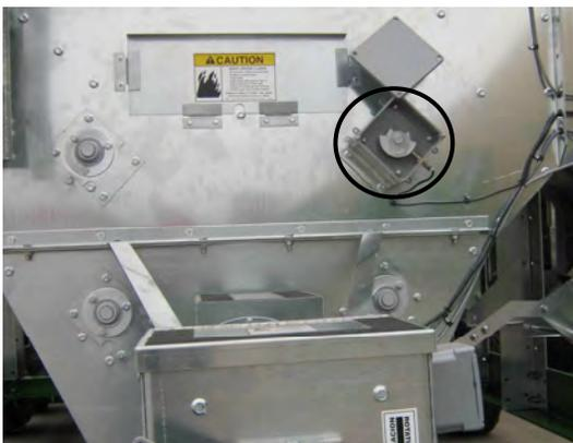
Figure 1.8c: Metering Roll Proximity Switch Installed on Dryer
