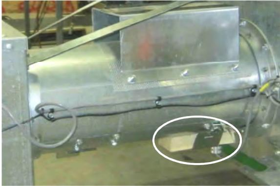
**Image 4-28 – Discharge moisture sensor installed**
