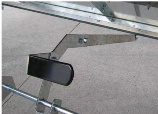
Image 29 – Unload auger cleanout door cam lock
