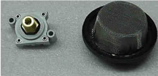
Figure 1.9b: Static Air Pressure Sensor Apart
