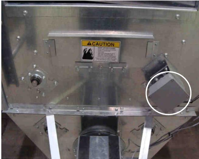
Image 4-18 – Meter roll proximity switch box
