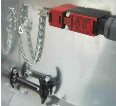
The main body of the switch is mounted next to door, with interlock key and chain attached to the door. Key must be removed from switch before door may be opened. If key has been removed from switch, a fault will be displayed and dryer will not start.
