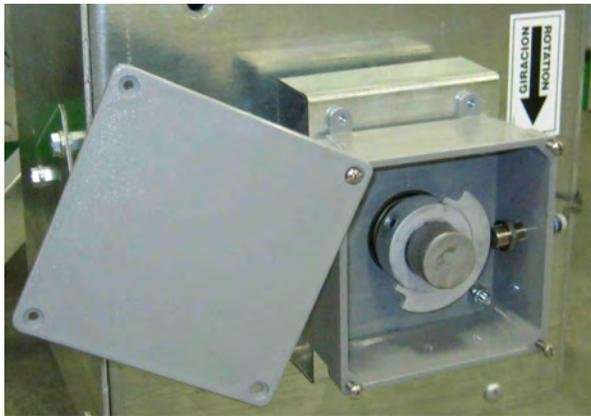
Image 15 shows unload auger proximity switch (at right in box) and rotating target.
