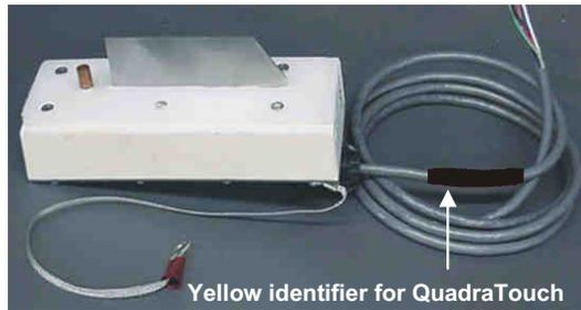
The Discharge Moisture sensor is found under the discharge chute at the rear of the dryer. It is used to calculate the moisture and temperature of the grain as it is discharged from the dryer.
