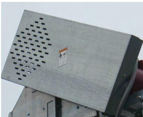
Image 42 – Load auger shield
