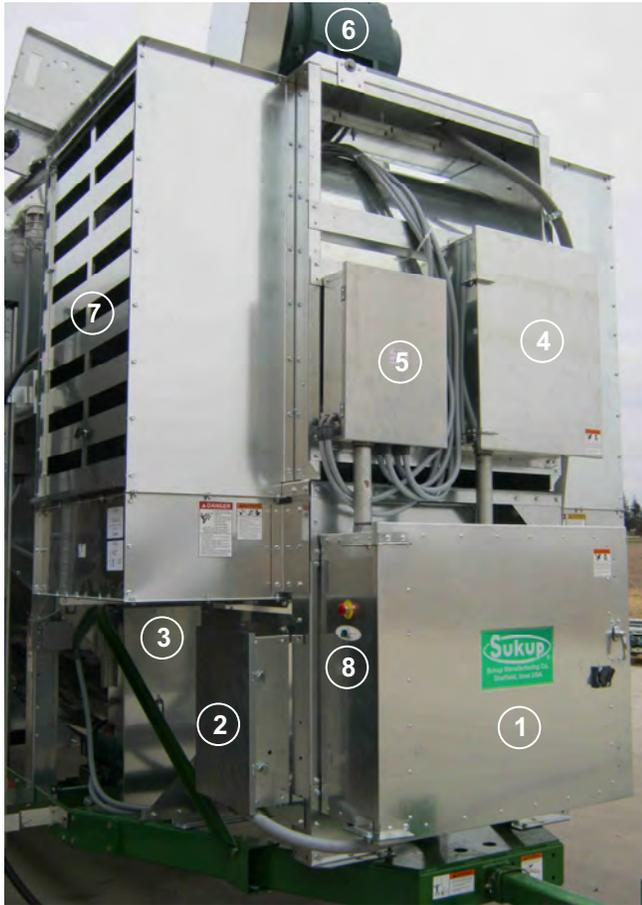
Image 4 – Front of Centrifugal Dryer
