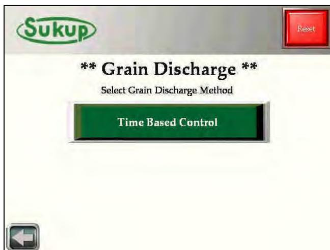
After selecting "Time Based Control" the computer will calculate a recommended dry time based upon the user's set points. That number is placed in the BLACK box. It is automatically loaded into the GREEN box, which is user selectable.
