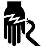
Mains Isolater must be located outside of bin. It must be easily accessible from ground level and must be lockable in off position. Mark clearly as to equipment it operates. See Mains Isolater decal placement information later in this section.
