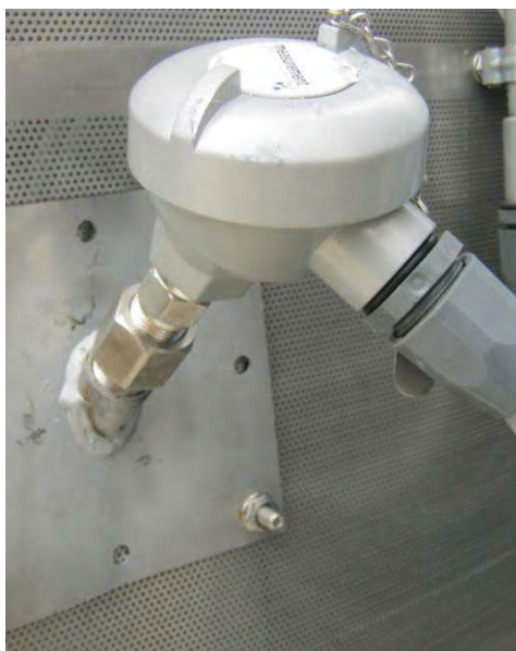
Image 11 – Single-point grain temperature sensor RTD
