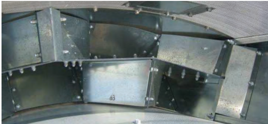
Image 14 shows grain exchangers, viewed from top.
