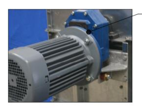
Transmission is pre-installed by manufacturer.
