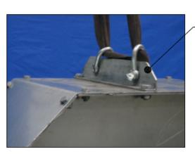
1. Lift bracket for elevator top The lift bracket allows the elevator to be liftet in order to install pipes under the top and the bottom under the pipes
