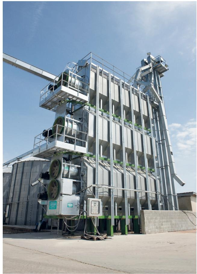
2 module stack dryers with capacities up to 78 t/h
